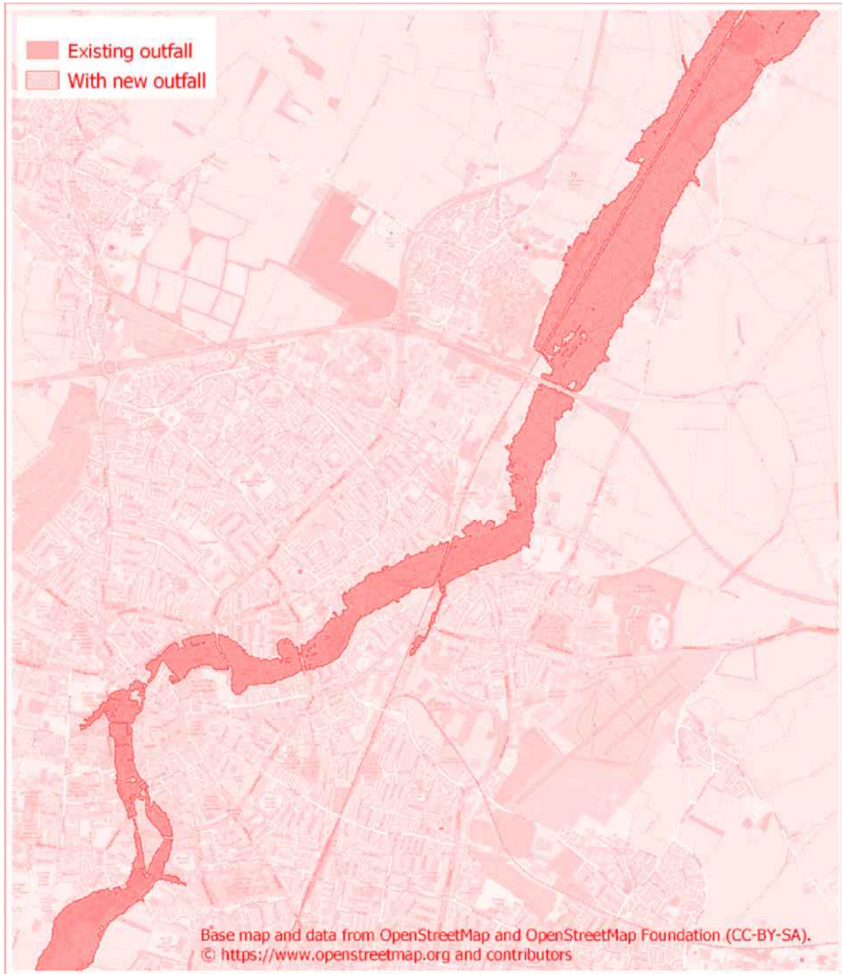
Figure 4.3. Sensitivity test – 1 in 100 year plus climate change, 61 hour storm, 15 hour outfall flow offset
