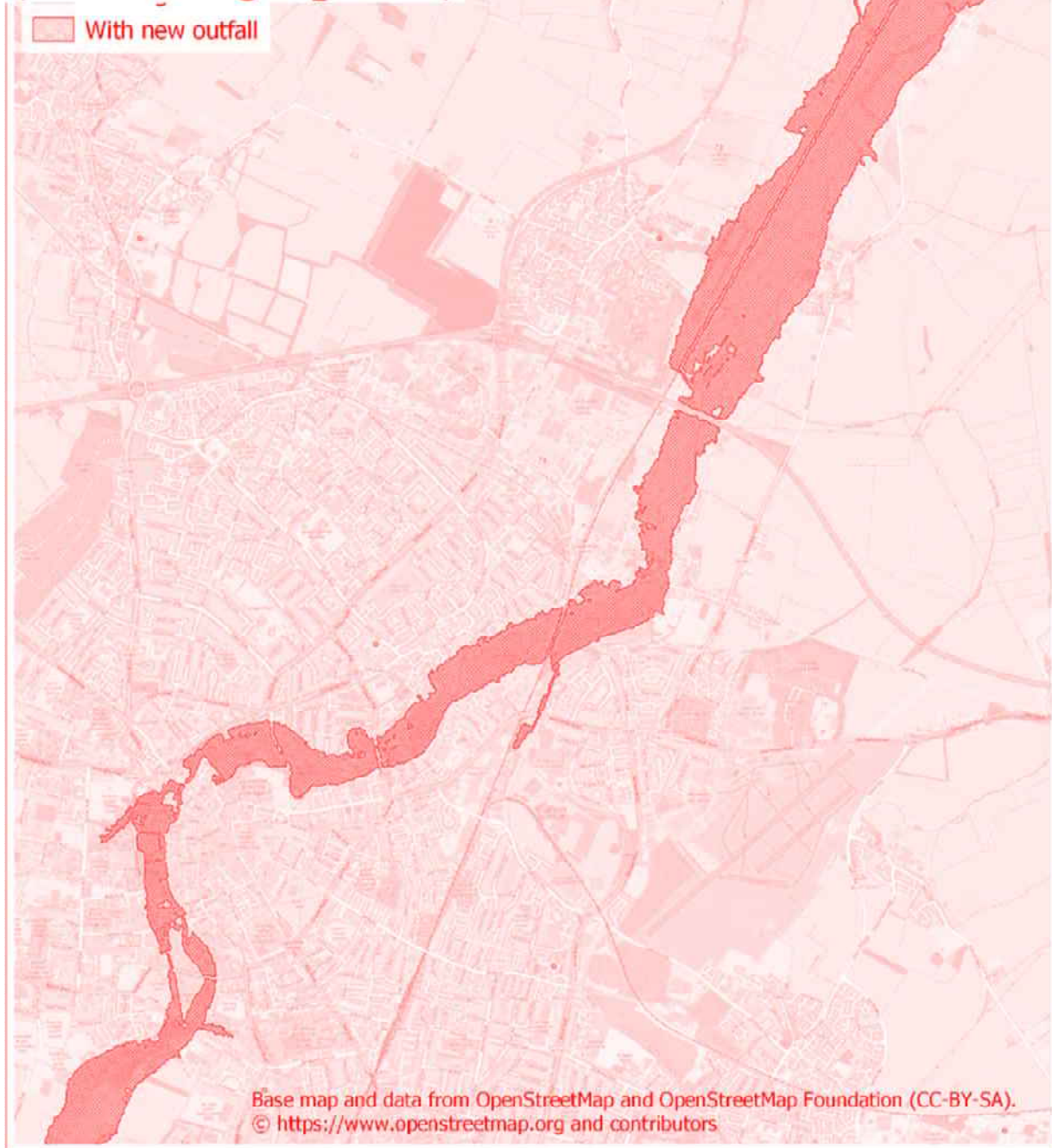
Figure 4.1 Table 6-2. Base case – 1 in 100 year plus 9% climate change, 61 55-hour storm, 30 hour outfall flow offset 1D model results
